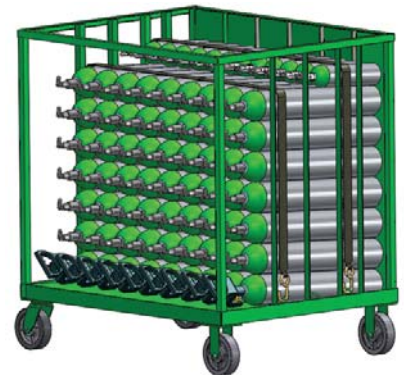
Part No. 9026 Holds 72 E or 132 M6 cylinders. Will hold 264 M6 cylinders (end to end). Deep enough to hold Grab 'N Go. Equipped with 6" rubber casters (2 rigid and 2 swivel-locking) and two 10 ft. ratchet straps with hooks. Solid floor. Powder coated green. Dim: 45.875"Hx34"Wx42.125"L
