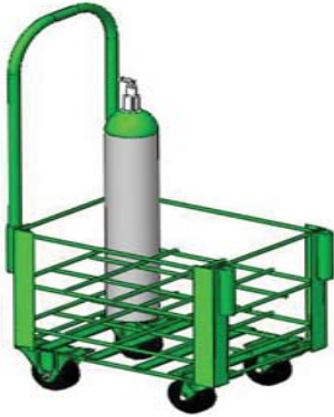
Part No. 1075HD Model: DE-12 HD Dim: 43"Hx15.5"Wx24.5"L 4" casters, 2 rigid & 2 swivel Holds 12 D/E/C/M7 or ML6 Cyl
