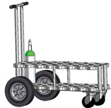
Part No. 2080 Model M6-24 Holds 24 M6 Cylinders Dim: 36.75"Hx16.5"Wx32"L Removable handle Zinc Plated
